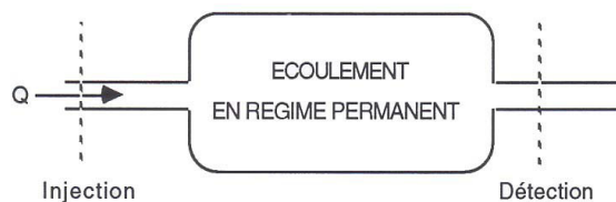
Fig. 4-1. General principle of radiotracer application in industry.
